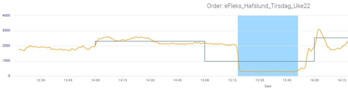
Figure 19 One test dispatch from the Hafslund/Elvia pool – combined portfolio of both industrial and commercial (building) loads. Tested in May 2020. Approx 1.75MW of flex (Screenshot by Enfo).
