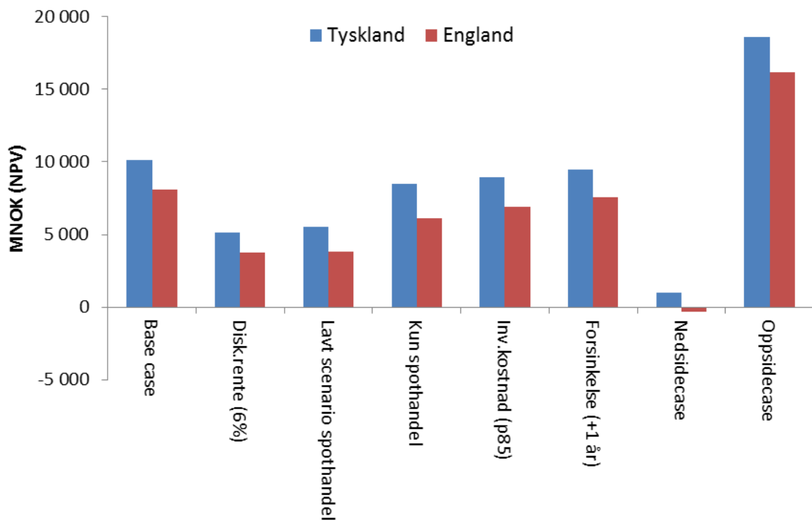
Figure 9: Summary of the uncertainty analysis (NPV as function of: 1 - Base case, 2 – Discount rate = 6 %, 3 – Low scenario for congestion revenues from day-ahead trade, 4 – Only revenues from day-ahead trade, 5 – Investment cost = p85, 6 – Delayed operation = 1 year, 7 – Downside scenario, 8 – Upside scenario).
