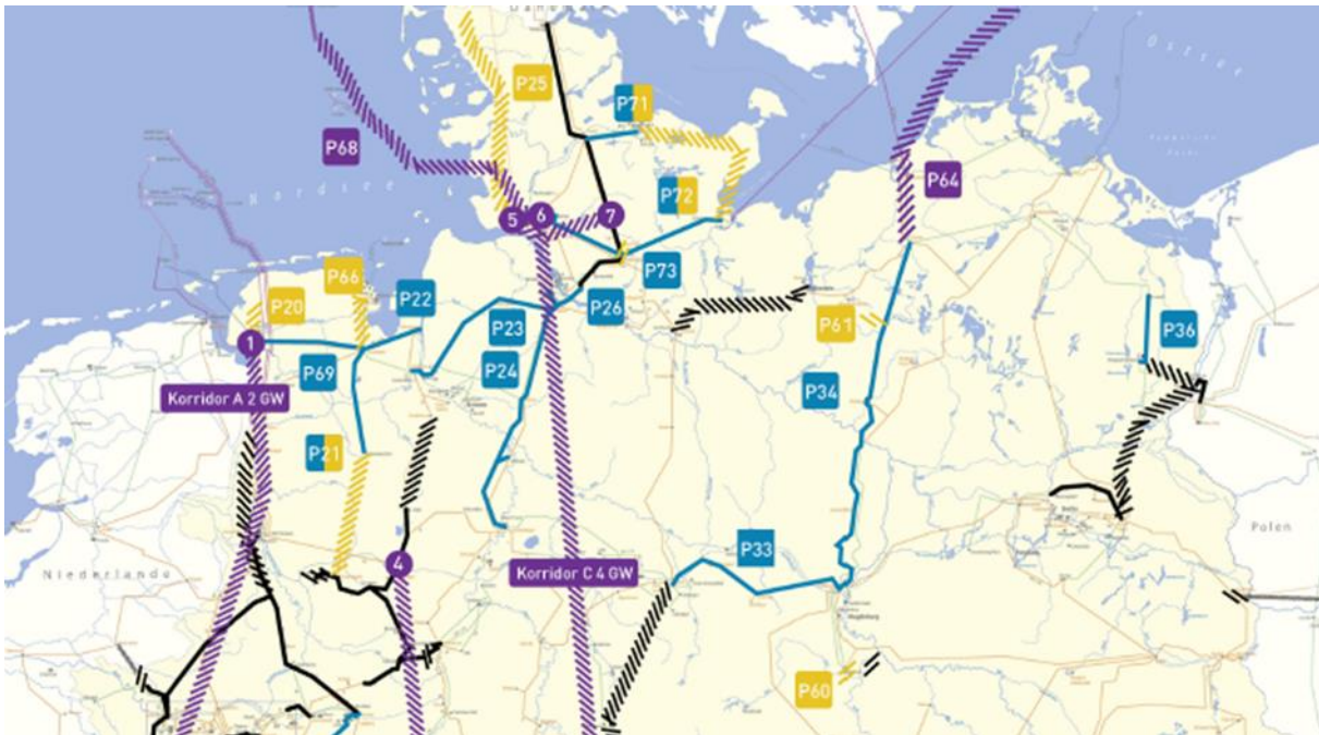
Figure 15: General map of planned HVDC interconnectors in the Hamburg area. 5 = Brunsbüttel, 6 = Wilster, 7 = Kaltenkirchen
