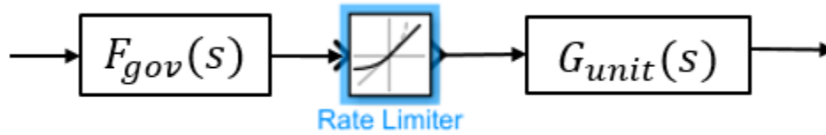
Figure 33. Block diagram of a unit with rate limit.
