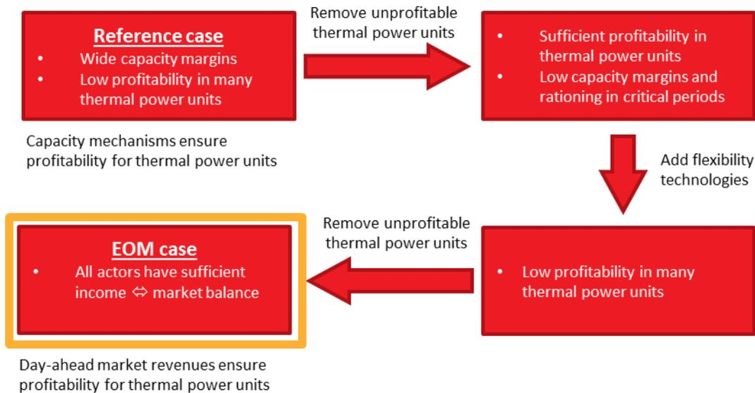
Figure 5. The energy-only market case (EOM) is constructed through a stepwise approach of adding flexibility technologies and removing thermal production units until prerequisites are fulfilled.
