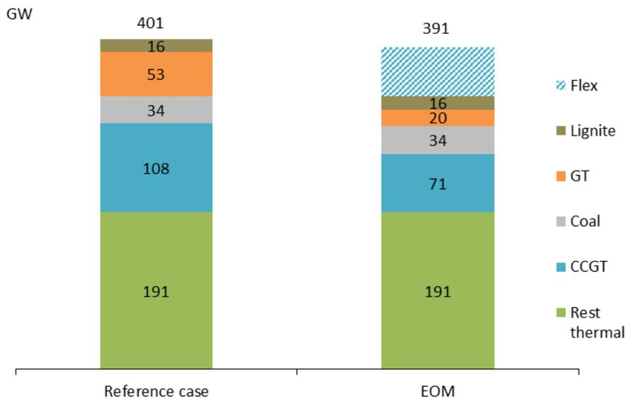
Figure 10. Installed thermal power and flexibility in Europe, comparison between our reference scenario and our scenario with energy-only market (EOM).
