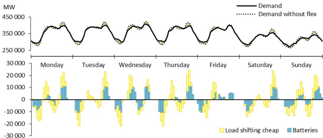
Figure 19. Contribution and effects of low-cost load shifting and batteries for Europe during a typical winter week in the energy-only scenario.
