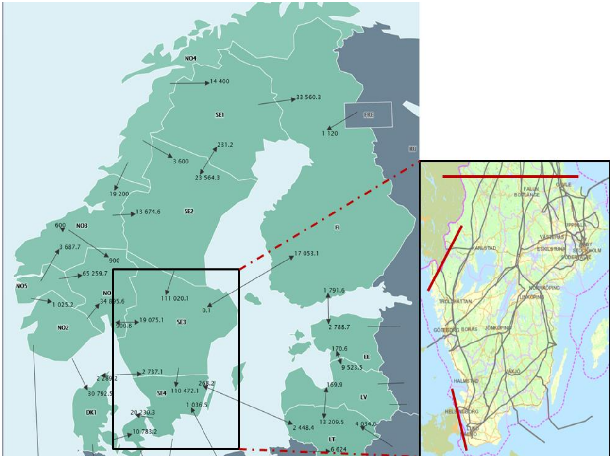
FIGURE 18. SCHEMATIC DESCRIPTION OF WHICH TIE-LINES MEASURED TO ESTIMATE GENERATION-LOAD IMBALANCES. MEASURED CUTS ARE THOSE SHOWN WITH A RED LINE IN THE MAP ON RIGHT HAND SIDE.
