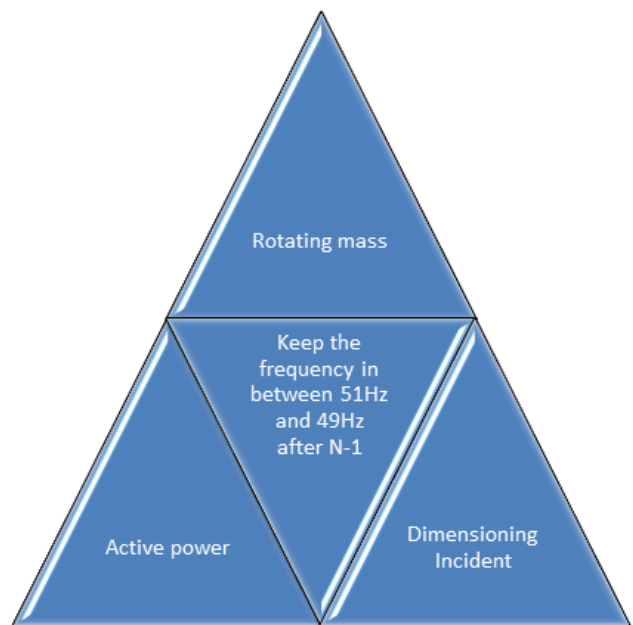
Figure 6 ‘Dials’ to keep 49 \text{ Hz} < f < 51 \text{ Hz} after an N-1 event
