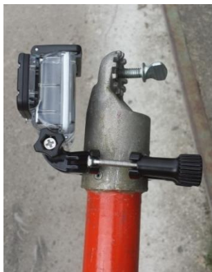
Installation of camera on insulation rod.
