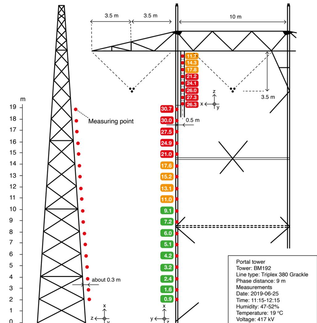
Measured electric field strength E [kV/m] for a 420 kV portal tower.
