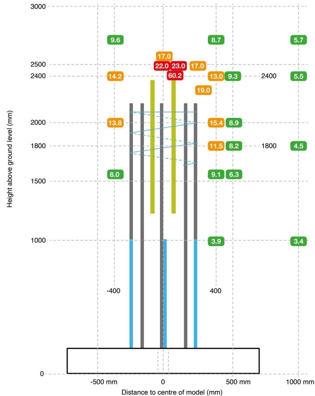
Measured electric field strength  $E$  [kV/m] around a model of a foundation with steel reinforcement and bolts.
